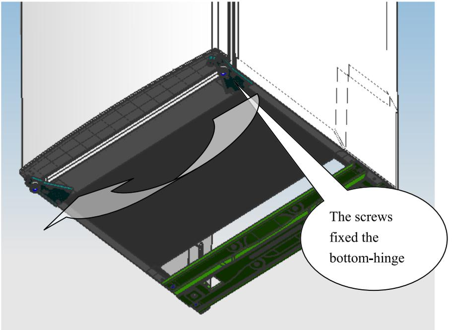
5、replace the leveler to the other side and adjust it to make sure the cabinet level
