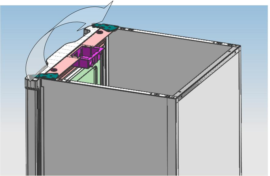
B、replace the door bearing bush and the limit block.
